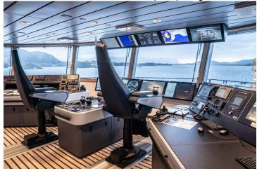
Navigation System consisting of ten Multipilot Platinum Navigation workstations, four Datapilot Platinum information display, a 55" Planning station, a dual Trackpilot Platinum integrated track steering system, Dynamic Positioning System, Sound Reception System, uninterruptable power system (UPS), a weather station, Voyage Data Recorder, Bridge Alarm Management and Bridge Navigational Watch Alarm System (BNWAS).
