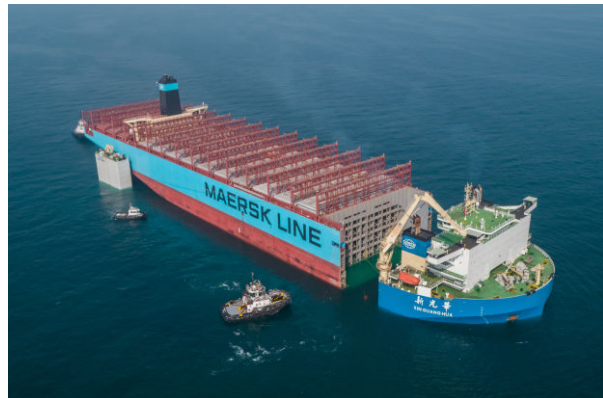
The undamaged portion of the Maersk Honam was loaded on to a semi-submersible ship and carried to South Korea where it will be rebuilt. Photo: Maersk Line
