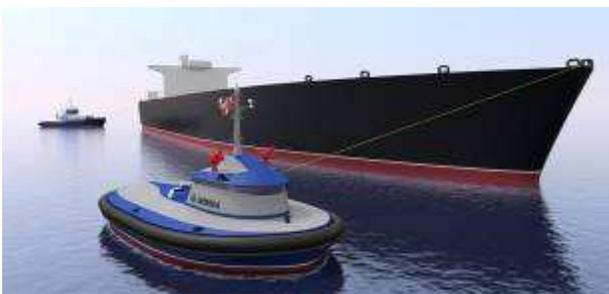
tug concept. The hull form, designed for high stability and good seakeeping performance in waves, is the product of extensive development work including CFD and towing tank testing. However, being a TOWBoT, with no need for a conventional wheelhouse, crew accommodation, domestic systems or lifesaving equipment, RAMora is claimed to be simpler and more compact than any conventional tug of comparable performance.
